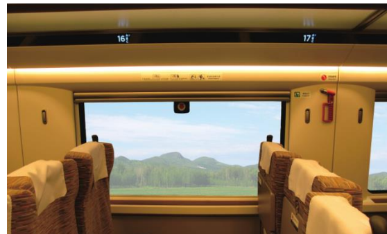
Emergency Escape Window and Emergency Hammer
